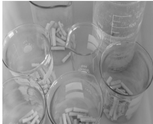
Fig.1.1 Appearance of analytical balance PRL TA14 and test samples during the water absorption test
