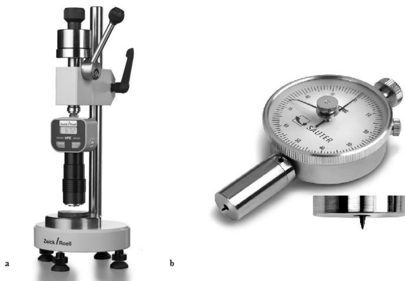
Fig. 2.1 Devices for measuring the hardness with the use of Shore method, a –Zwick 3130, b - Sauter HTB 100
