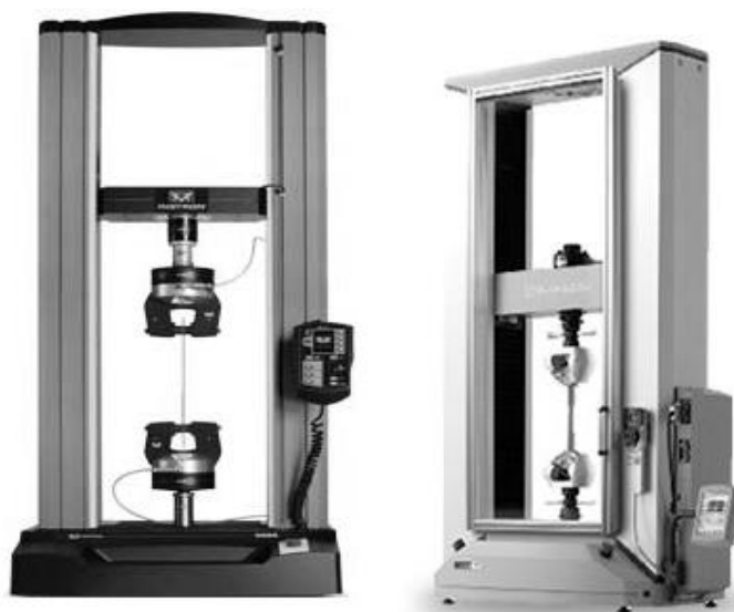
Fig. 3.1. Two-column strength testing machines manufactured by: a) Instron, b) Shimadzu [www.instron.com, www.shimadzu.com]
