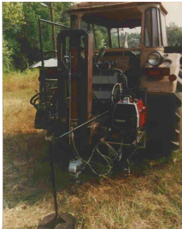
Fig.1.2 Bewameter for traction tests of soil properties (WITPiS Sulejówek)
