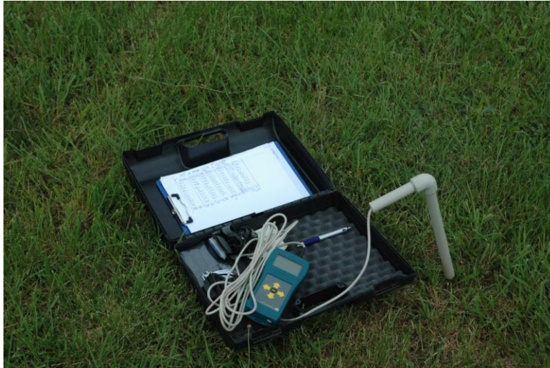
Fig. 3.3 FOM gauge in a set for field measurement
